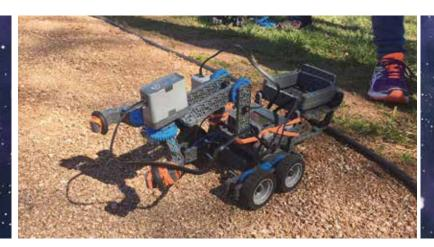
After spending a significant amount of time programming, our rover was quickly dispatched by a hill—because its center of the balance did not easily allow for climbing. We learned that accounting for circumstances we cannot control is as important as designing the parameters we can control.
