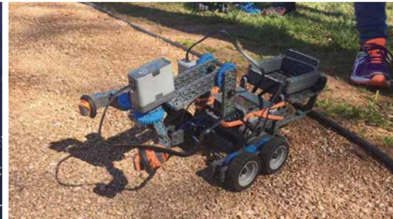
*After spending a significant amount of time programming, our rover was quickly dispatched by a hill—because its center of the balance did not easily allow for climbing. We learned that accounting for circumstances we cannot control is as important as designing the parameters we can control.*
